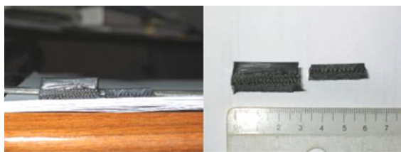
Fig. 20 Pictures of tyre sections: Lab 1 ( thick tyre on the left side of both pictures ) and Lab 2 ( thin tyre on the right side of both pictures )
