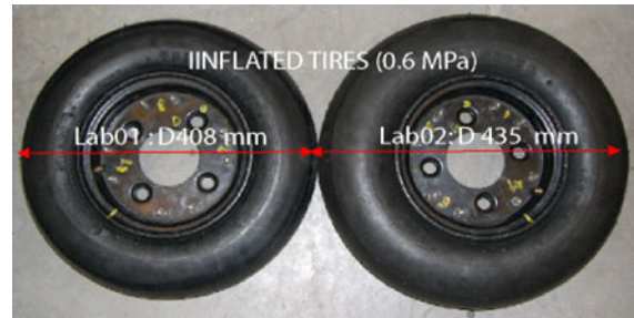
Fig. 19 Tyres size comparison between Lab 1 and Lab 2
