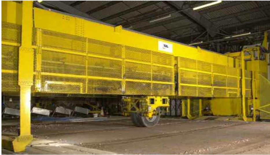
Figure 4. The TRL Pavement Testing Facility (Crowthorne, UK)
