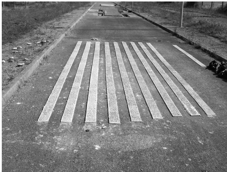
Figure 2. Testing site for the cracking strips (tests performed at LCPC Nantes).
