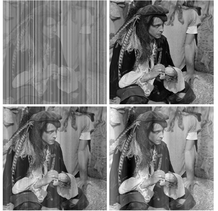
Fig. 5. Top-left: noisy pirate. Top-right: denoised using VSNR. Bottom-left: denoised using DeStripe [8]. Bottom-right: denoised using Wavelet-FFT [18]. This experiment corresponds to the last line of Table I. The noise pattern is a vertical line. The DeStripe and Wavelet-FFT algorithms do not completely remove low frequencies while VSNR leads to near perfect results.
