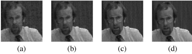
Fig. 8. Output of filtered Trevor White third frame 256 \times 256 corrupted by mixed impulsive ( p = 5\% ) and Gaussian additive noise ( \sigma = 20 ): (a) 3-D NLMS L -filter with ( \mu_0 = 0.8 ), (b) 3-D recursive NLMS L -filter with ( \mu_0 = 0.8 ), (c) 3-D NLMK L -filter with ( \mu_0 = 10^{-4} ), and (d) 3-D recursive NLMK L -filter with ( \mu_0 = 10^{-4} ).
