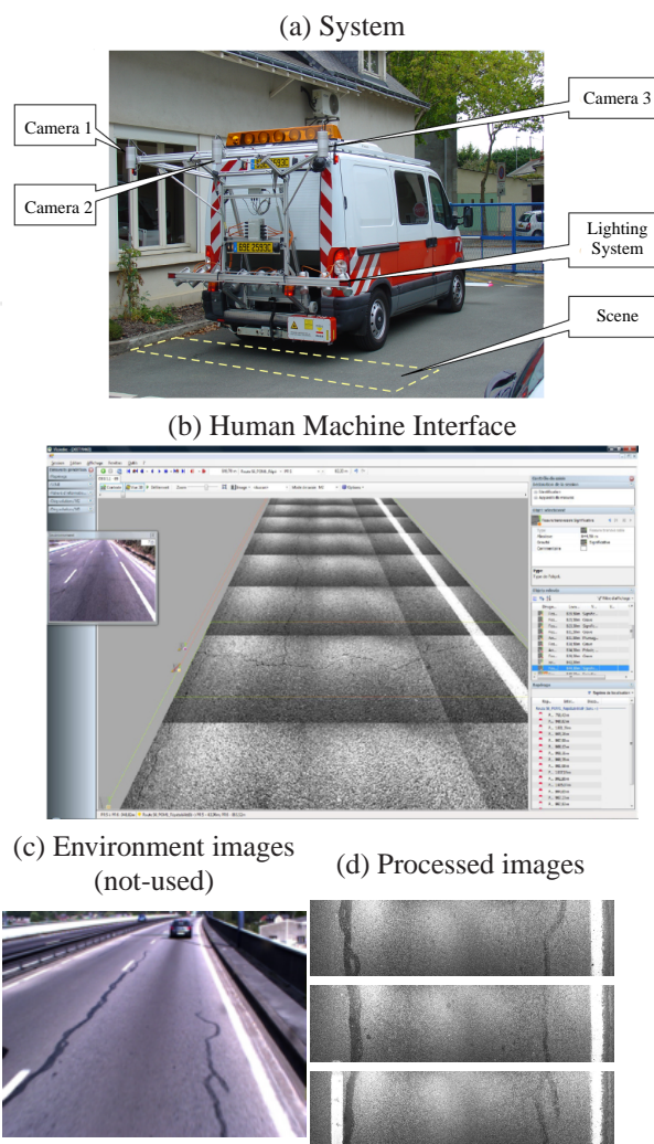
Figure 6: The acquisition system used for the evaluation – In (a), The acquisition system is illustrated. In (c) and (d), an example of the final images is given. In (d), we can see the road that is visible in (c). The processing is done 1 meter by 1 meter, i.e. independently on each image presented in (d). The surface contains two reparations of vertical cracks. In some cases, the sensors do not have the same settings and the global illuminations are different, so, it can generate some “false cracks”. This aspect has been easily taken into account in a pre-processing step by eliminating the junction area in the region of interest.
