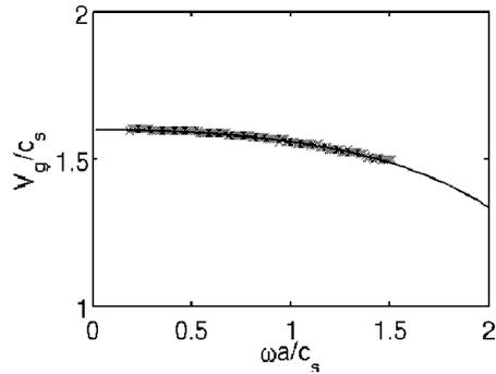
Figure 13: Central wire (cylindrical). Normalized group velocity vs. frequency measured with the magnetostrictive device (x-mark) and computed with the SAFE model (solid line) for the  $L(0,1)$  mode.
