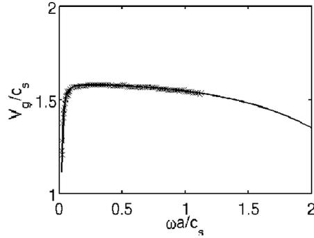
Figure 14: Peripheral wire (helical). Normalized group velocity vs. frequency measured with the magnetostrictive device (x-mark) and computed with the SAFE model (solid line) for the  $L(0,1)$  mode.
