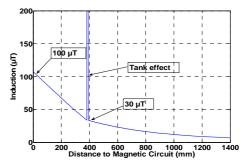
Fig. 5. Induction outside the magnetic circuit (Path 1)
