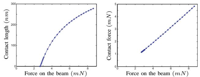
Fig. 2. Results of the semi-analytical structural contact model
