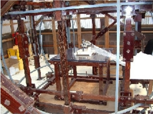
Fig. 9 SCM placed at the center of three Helmholtz coils that generate the test magnetic field. A set of other coils cancel the effect of the earth's magnetic field
