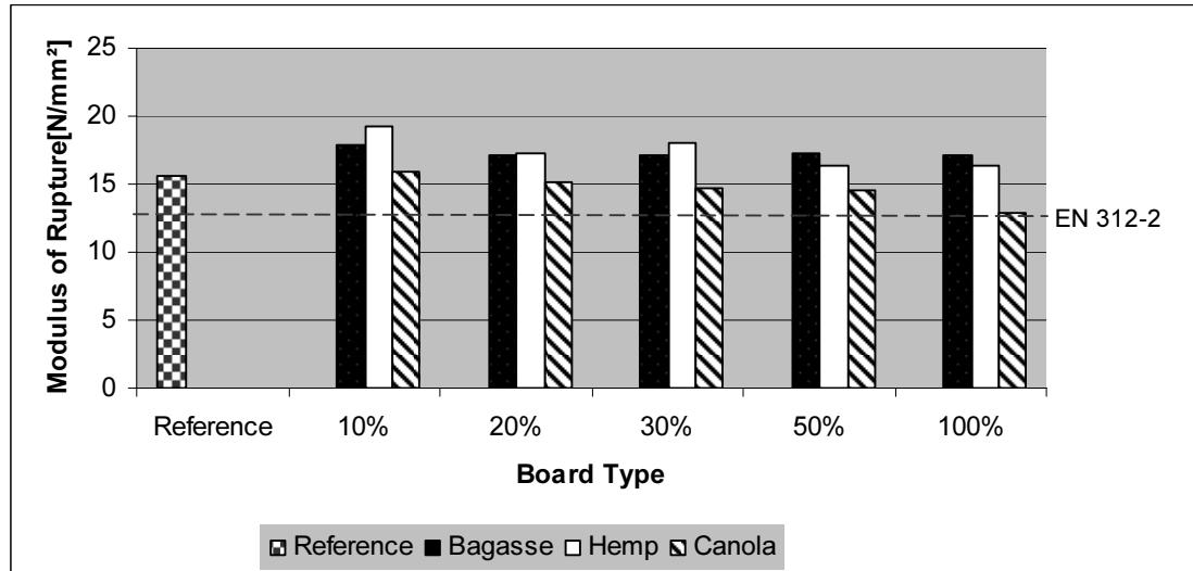
Figure 2: Comparison of bending modulus of particle boards, containing bagasse, hemp and canola, each in mixture with wood in the middle layer
