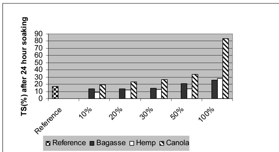
Figure 5: Comparison of water absorption of particle boards, containing bagasse, hemp and canola, each in mixture with wood and references after 24 hour soaking
