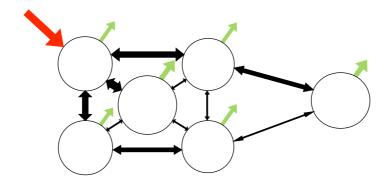
**Figure 4.** Entropy repartition over the sub-systems. Red arrow, injected entropy rate; Black arrow, mixing entropy rate; Green arrow, dissipated entropy rate; Black circle, sub-system entropy
