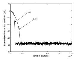
**Fig. 4.** Comparison of convergence of the SCR2 adaptive algorithms for the three-channel system at 50 dB SNR with different channel order.
