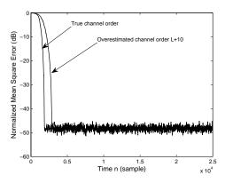
**Fig. 3.** Comparison of convergence of the SCR2 adaptive algorithms for the three-channel system at 50 dB SNR with the true channel order and overestimated channel order.
