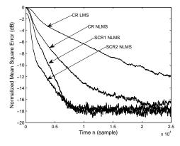
**Fig. 1.** Comparison of convergence between the CR and SCR adaptive algorithms for the three-channel system at 20 dB SNR.
