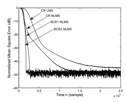
**Fig. 2.** Comparison of convergence between the CR and SCR adaptive algorithms for the three-channel system at 50 dB SNR.
