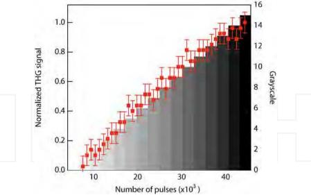
Fig. 5. THG signal versus number of the laser pulses with I = 6 TW.cm<sup>-2</sup>. The information can be grayscale encoded.
