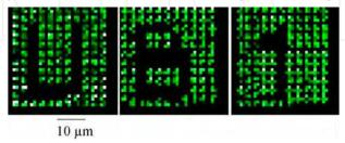
Fig. 4. THG readout of the three layers containing the bit patterns U, B, and 1, recorded in the bulk of the glass (bit spacing, 3 mm; layer spacing, 10 mm). Laser writing parameters:  $I = 6 \text{ TW.cm}^{-2}$ ,  $N = 10^6$ . The three THG images present high signal-to-noise ratio and no cross talk.
