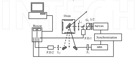
Fig. 11. Nanosecond time resolved pump-probe set-up.
