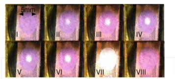
Fig. 9. (I) and (VII) colour of the sample in the LS state. Evolution of the sample set in the thermal hysteresis loop and impacted by (II) one pulse, (III) two pulses, (IV) three pulses, (V) four pulses, (VI) five pulses. (VIII) Colour of the sample impacted by five laser pulse and cooled back in the LS state.
