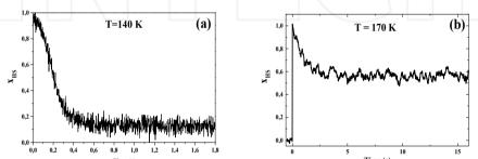
Fig. 7. HS  $\rightarrow$  LS relaxation curves (a) At 140 K below the hysteresis loop. The sample was firstly cooled down to a pure LS state and then carefully warmed
