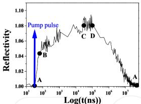
Fig. 13. Time dependence of the reflectivity change at 283 K after photo-excitation with a pump pulse of fluence  $E_p \sim 9$  mJ.cm<sup>-2</sup>.
