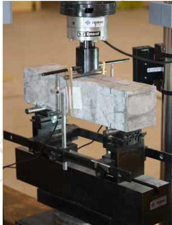
Fig. 1. (a) Schematic diagram and (b) photo of experimental set-up for three-point bending tests on beams.
