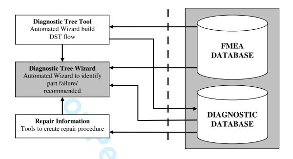
Figure 10. DST Application Structure
