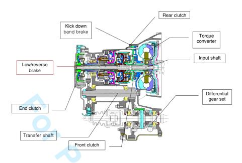
Figure 1. Sectional View of KM series Automatic Transmission
