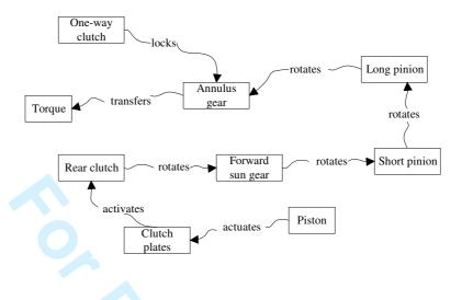
Figure 8. Functional Diagrams for 1<sup>st</sup> Gear (D, 2, L range)
