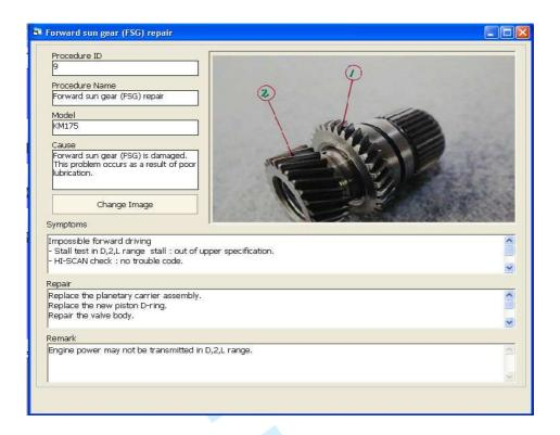
Figure 11. Repair Procedure for Sun Gear
