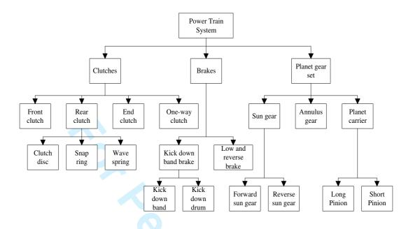
Figure 6. Structural Decomposition of Power Train System
