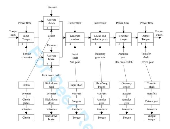
Figure 7. Function and Structure Mapping (Based on FMAG Approach, Teoh 2003)
