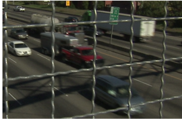
Damaged AVC video after concealment (buffer repetition)
