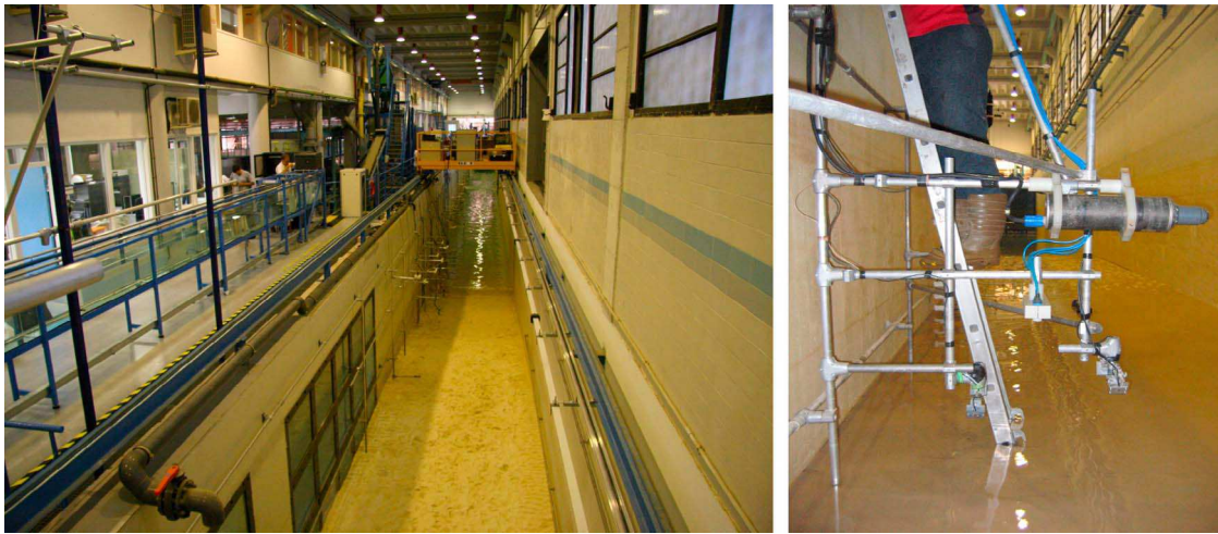
Figure 1. Photographs of (left) the 100 m long, 3 m wide, and 5 m deep wave channel at UPC-CIEM, Barcelona, Spain, and (right) the experimental arrangements of the instruments.
