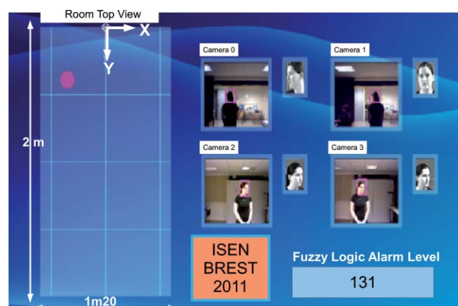
Fig. 14 User interface of the fuzzy logic and optical correlation-based face-recognition method developed using Matlab software and a CPU: Intel Dual Core E5300, 2.6 GHz, 2Go RAM computer. (Color online only.)
