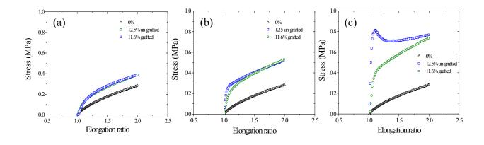
Figure 8: Stress as a function of elongation ratio: direct comparison between grafted ( $\bigcirc$ ) and un-grafted ( $\square$ ) cases: from the lowest silica volume fractions ((a), 4.00% un-grafted 4.30% grafted) to higher volume fractions ((b), 7.50% un-grafted, 8.10% grafted, and (c), 12.50% un-grafted, 11.60% grafted). Each time the stress curve for the pure polymer is also plotted ( $\Delta$ ).
