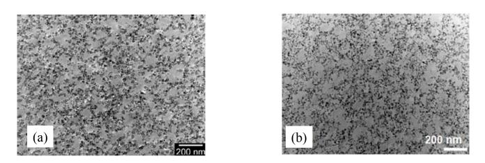
Figure 6: (a) TEM picture of the un-grafted nanocomposite filled with 15.40 % v/v of silica particles (black is silica and grey is polymer). (b) TEM picture of the grafted nanocomposite filled with 11.60 % v/v of silica particles.
