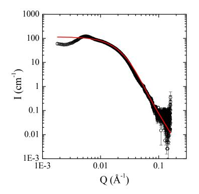
Figure 1: SAXS curve of a diluted solution (0.1% v/v) of native silica particles dispersed in DMAc. The full red line is the result of the fit with a polydisperse spheres form factor with a mean radius R = 6 nm and a polydispersity  $\sigma_{\text{log-normal}} = 0.3$ .
