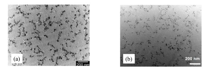
Figure 4: (a) TEM picture of the un-grafted nanocomposite filled with 6.65 % v/v of silica particles (black is silica and grey is polymer). (b) TEM picture of the grafted nanocomposite filled with 4.30 % v/v of silica particles.
