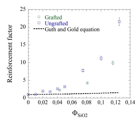
Figure 9: Relative reinforcement from stress/strain curves as a function of silica volume fraction for grafted ( $\bigcirc$ ) and un-grafted ( $\square$ ) silica nanocomposites. The black dash line corresponds to the Guth and Gold predictions for spherical fillers.
