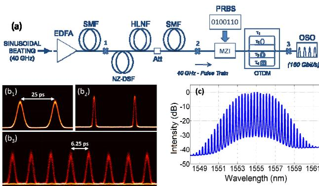
Fig. 4. (a) Experimental setup used to generate low duty-cycle pulse trains at 40 GHz and 160-Gbit/s PRBS OTDM signal. (b<sub>1</sub>), (b<sub>2</sub>) and (b<sub>3</sub>): Intensity profiles of the pulse train at points 1, 2 and 3. (c) Optical spectrum at point 3.
