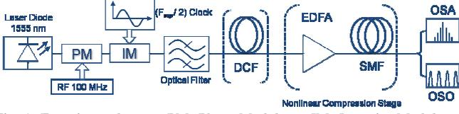
Fig. 1. Experimental setup. PM: Phase Modulator, IM: Intensity Modulator, DCF: Dispersion Compensating Fiber, EDFA: Erbium Doped Fiber Amplifier, OSA: Optical Spectrum Analyzer, OSO: Optical Sampling Oscilloscope.
