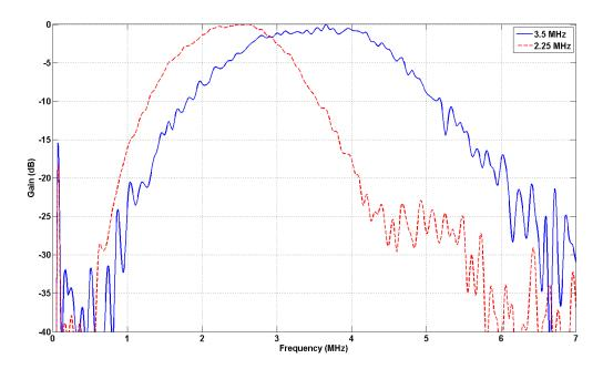
Figure 2. Bandwidth of transducers.
