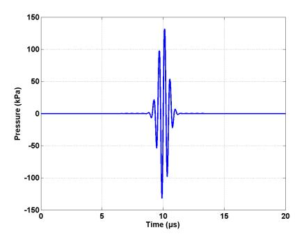
Figure 1. Emission signal with 4 cycles.
