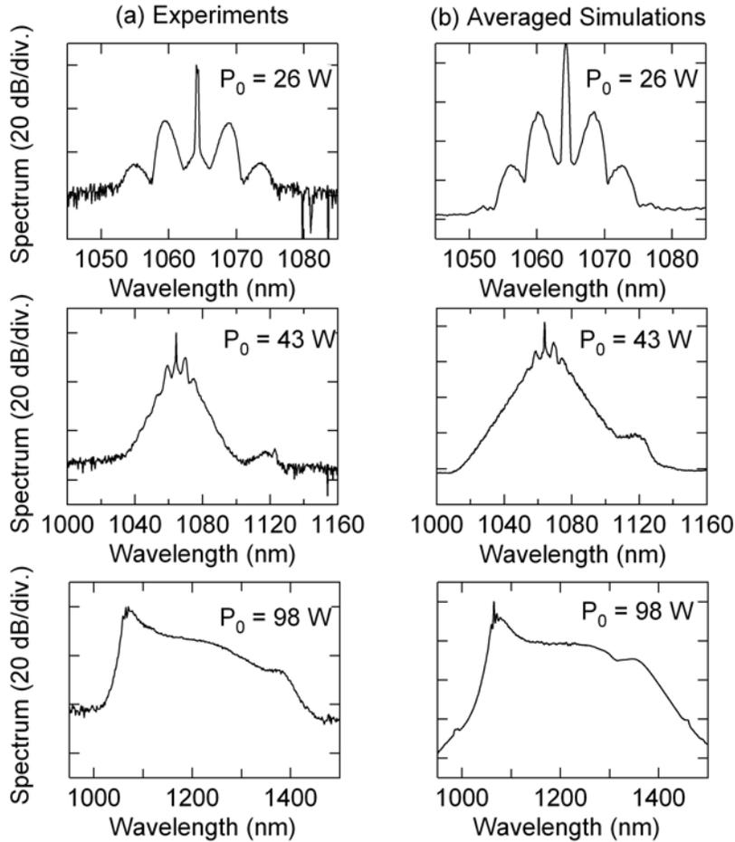
**Fig. 1** Experimental results (left) and numerical simulation results (right) for 1 ns pulses at 1064 nm injected into highly nonlinear PCF at peak powers as shown. Note that the simulation results are averaged and convolved with a spectral resolution function matching the bandwidth of the spectrum analyzer used in the experiments (0.1 nm for 26 W results; 0.4 nm for 43 W results; 1.6 nm for 98 W results) [10].
