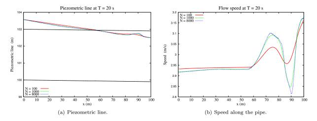
Figure 24: Piezometric line and speed along the pipe at time  $t=20\,s.$
