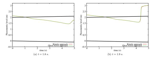
Figure 33: Water hammer test case in non uniform closed water pipe.
