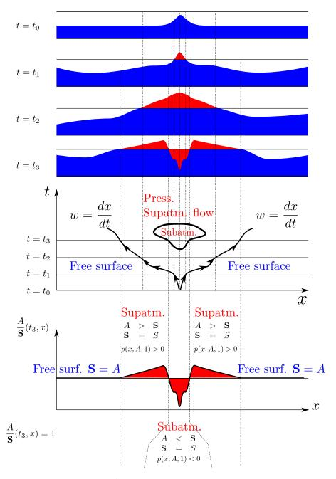
Figure 13:  $\frac{A}{S_w}$  criterion to detect depression area.
