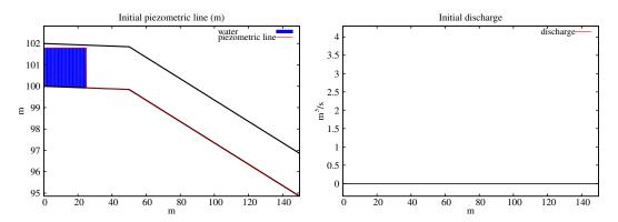
Figure 27: Piezometric line (left) and discharge (right) at initial condition.
