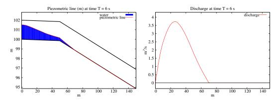
Figure 28: Piezometric line (left) and discharge (right) at time  $T=6\,s$ .
