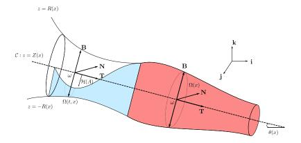
Figure 1: Geometric characteristics of the domain: free surface and pressurized flow.
