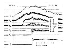
Figure 16: Wiggert: experimental data.  $y_2$ : upstream hydrograph,  $y_3$ : downstream hydrograph.  $h_A$ ,  $h_B$ ,  $h_C$ ,  $h_D$ : pressure head at 0.5 m, 3.5 m, 5.5 m and 9.5 m from the tunnel entrance (location of recording instruments) ([33]).
