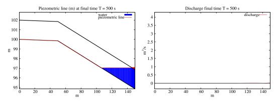
Figure 30: Piezometric line (left) and discharge (right) at final time  $T = 500 \, s$ .
