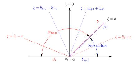
Figure 7: Pressurized state propagating downstream.
