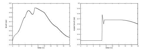
Figure 15: Wiggert's test: upstream hydrograph (up) and downstream water level (down).
