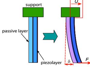
Fig. 2. Piezocantilever principle.
