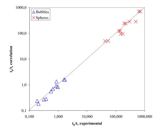
Figure 9. Parity diagram between the experimental and correlated values of  $t_p/t_c$  (Eq. 7).
