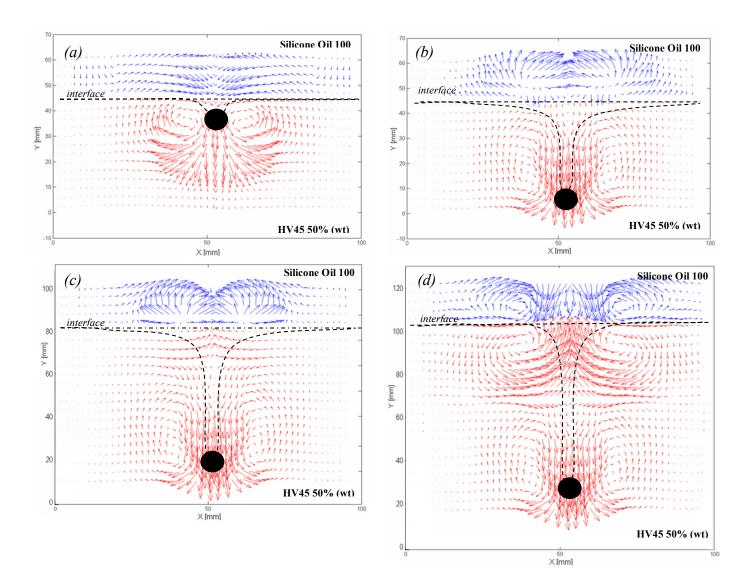
**Figure 8.** Flow fields around a 6 mm sphere diameter crossing an interface obtained by the PIV device. (a) t = 0.1 s, (b) t = 0.15 s, (c) t = 0.2 s, (d) t = 0.25 s after the interface contact.
