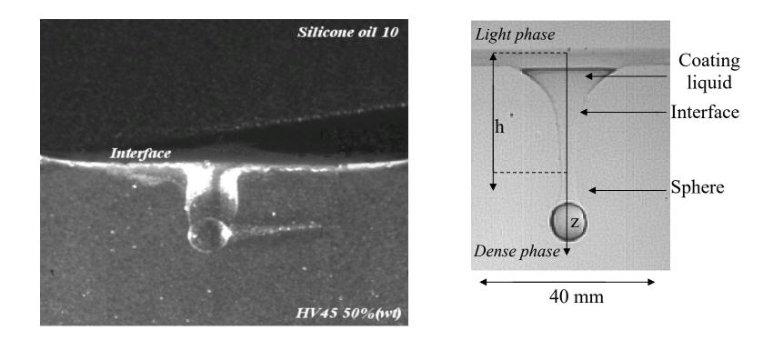
**Figure 6.** Example of images obtained by the PIV camera at the interface with seeding particles for Silicon oil 10 /HV45 50% system (reflection comes from the interface).
