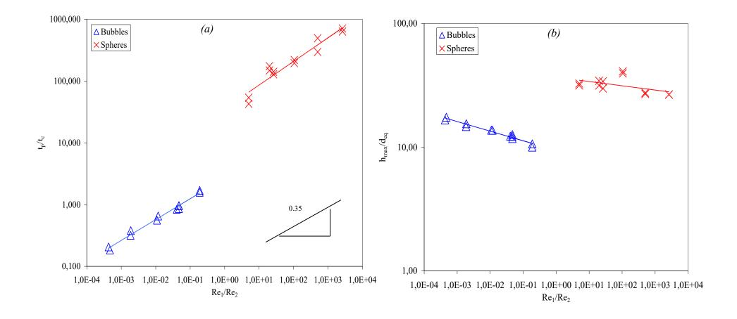
**Figure 5**. (a) Variation of the dimensionless passage time of the particles  $t_p/t_c$  in the various liquid-liquid systems studied in function of the ratio between two Reynolds numbers ( $Re_1/Re_2$ ). (b) Variation of the dimensionless height of liquid entrained behind the particle  $h_{max}/d_{eq}$  in these systems in function of Re<sub>1</sub>/Re<sub>2</sub>.
