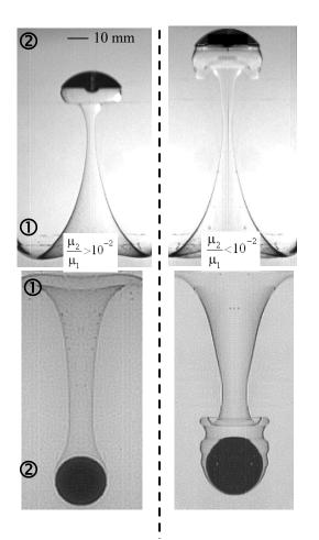
**Figure 11.** Hydrodynamic instabilities observed for the passage of both sphere and bubble. Phase 1 is the initial contact phase and phase 2 the second phase.
