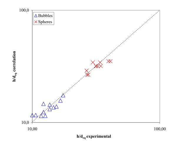
**Figure 10.** Parity diagram between the experimental and correlated values of  $h/d_{eq}$ .
