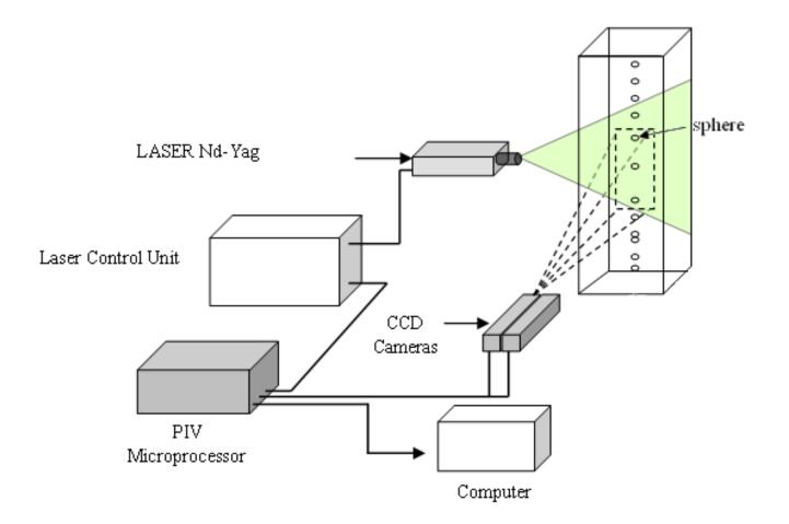
Figure 1. Set up of the Particle Image Velocimetry (PIV) system.
