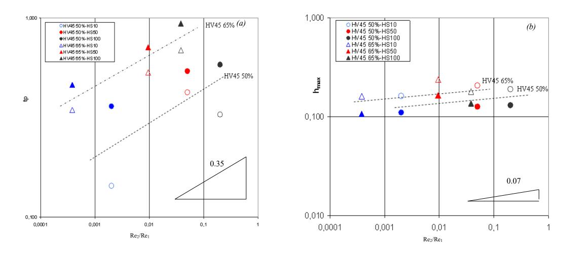
**Figure 4.** (a) Evolution of the passage time of spheres. (b) Evolution of the height of liquid entrained behind the sphere. Spheres of 4 mm (empty symbol) and 6 mm (full symbol) diameter at six different liquid-liquid interfaces composed by Silicone oil 10, 50 and 100 mPa.s as light phase and HV45 50% and 65% wt as dense phase. Dash line coresonf to the correlation established for each heavy liquid.
