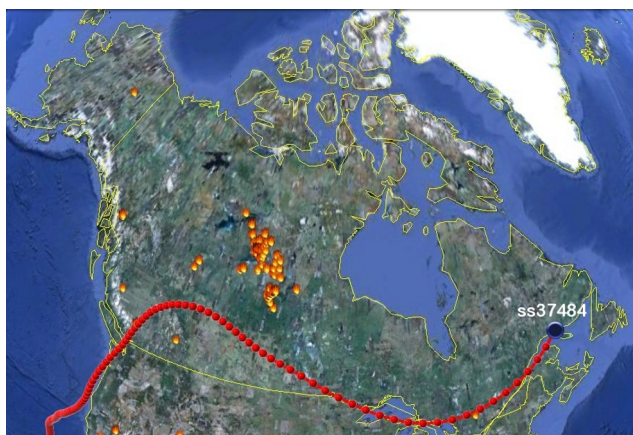
Fig. 1. A sample output of the trajectory data obtained using HYSPLIT. The 3-day back trajectory calculated from occultation ss37484 measured on 29 July 2010 is displayed in Google TM Earth with the instances of fire activity observed by MODIS over Canada on 27 July 2010. Spatial and temporal coincidences of the trajectory confirm that the emission source of the ACE-FTS measurement of enhanced HCN to be the widespread Boreal fires in northern Saskatchewan and parts of the Northwest Territories.
