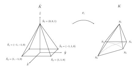
Figure 1: transformation F for a pyramid
