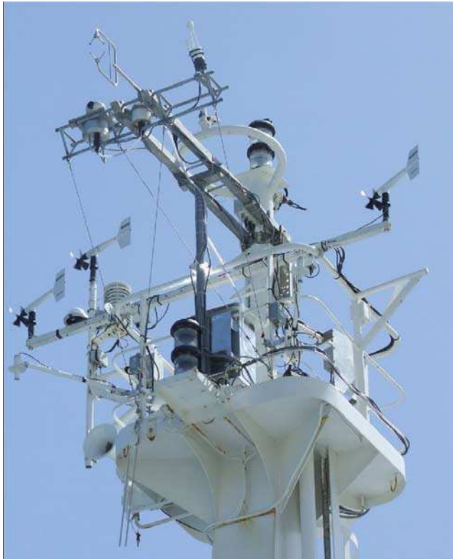
Figure 1. Overview of the flux measurement system, mounted on R/V Atalante .
