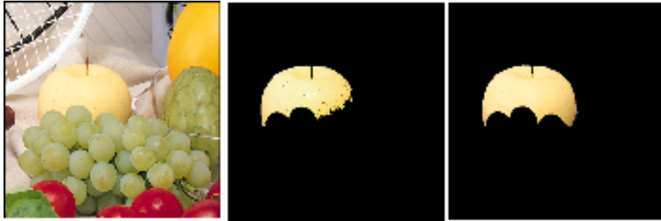
Figure 20: Left: initial image Center: result of the magic wand Right ; smallest region of the hierarchy containing the magic wand.
