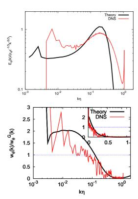
FIG. 2: DNS and theoretical results. Top: compensated scalar spectra in isotropic turbulence at a Taylor-scale Reynolds number of 427 and Sc=1. Bottom: comparison of the spectrum of the mean square advection term of the scalar equation in isotropic turbulence to its Gaussian value. In the inset the same results are plotted in linear representation.
