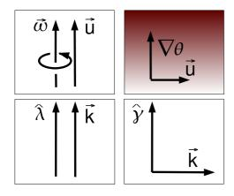
FIG. 1: Left, top: velocity Beltramization; bottom: depletion of nonlinearity through alignment of the Lamb-vector and the wavevector. Right: scalar Beltramization in physical and Fourier space.
