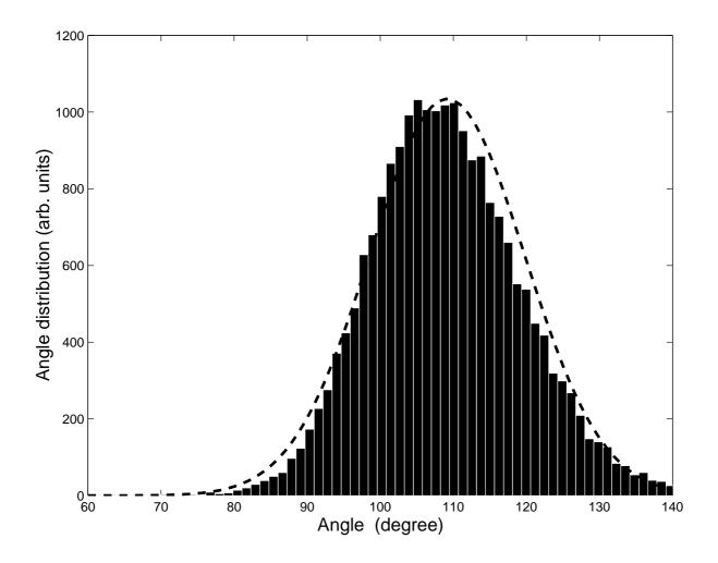
FIG. 2: Angular distribution in the a-Si cluster.
