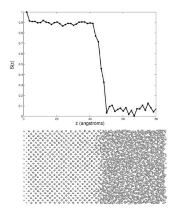
FIG. 6: Structure factor along the growth direction calculated for a stack of 8034 atoms. The structure factor and a representation of the atoms are aligned to evidence the link between the order/disorder and the value of the structure factor.
