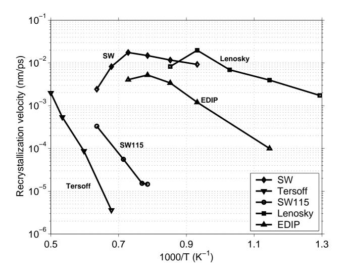
FIG. 8: Recrystallization velocity versus the inverse temperature for the 5 interatomic potentials.
