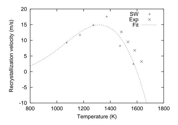
FIG. 11: Simulations of the recrystallization velocities with the Stillinger-Weber potential (+), measurement of the velocity of recrystallization of melted Si [38]  $(\times)$  and fit of the simulations according to Eq. 3.
