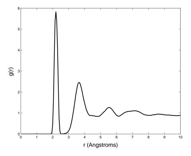
FIG. 3: Radial distribution in the a-Si cluster.
