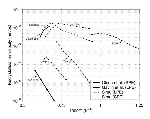
FIG. 17: Experimental and calculated velocities of recrystallization versus the temperature. The temperature has been rescaled for the simulations following  $T_{\rm rescaled} = T_{\rm simu} \times T_{\rm m,exp}^c / T_{\rm m,simu}^c$ , where the experimental melting temperature of c-Si  $T_{\rm m,exp}^c$  is equal to 1685 K and the simulated melting temperature of c-Si  $T_{\rm m,simu}^c$  is potential dependent.
