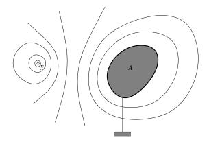
FIGURE 5. Green's function  $G_{A^c}(x, y)$  for Brownian motion is equal to the electrostatic potential in x created by a unit charge in y and a grounded conductor in A.
