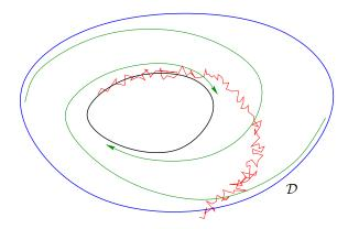
FIGURE 9. Two-dimensional vector field with an unstable periodic orbit. The location of the first exit from the domain  $\mathcal{D}$  delimited by the unstable orbit displays the phenomenon of cycling.
