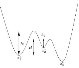
FIGURE 7. Example of a three-well potential, with associated metastable hierarchy. The relevant communication heights are given by  $H(x_2^*, \{x_1^*, x_3^*\}) = h_2$  and  $H(x_1^*, x_3^*) = h_1$ .
