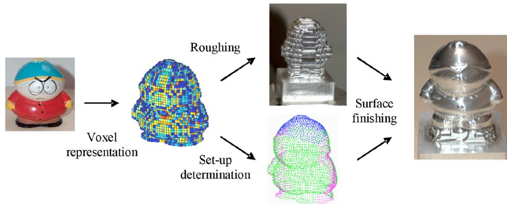
Figure 13. Direct duplication in 5-axis discrete machining.
