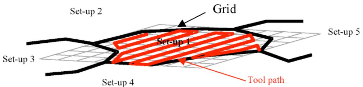
Figure 12. Machining area by set-up
