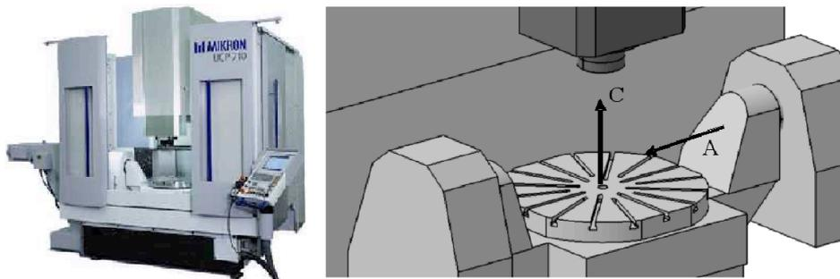
Figure 8. 5-axis machine tool (RRTTT structure)
