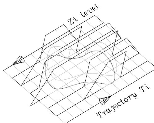
Figure 2. Resulting roughing trajectory
