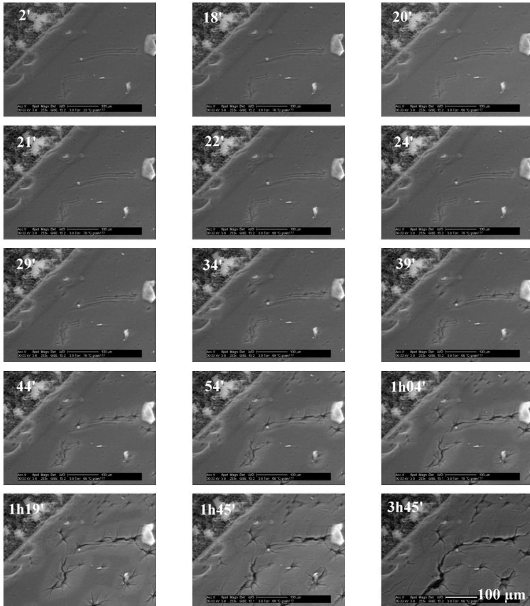
Fig. 6. Views of a  $\text{Li}_2\text{SO}_4\cdot\text{H}_2\text{O}$  single crystal during dehydration with the environmental scanning electron microscope ( $T=70^\circ\text{C}$ ,  $P(\text{H}_2\text{O})=5.2$  hPa).
