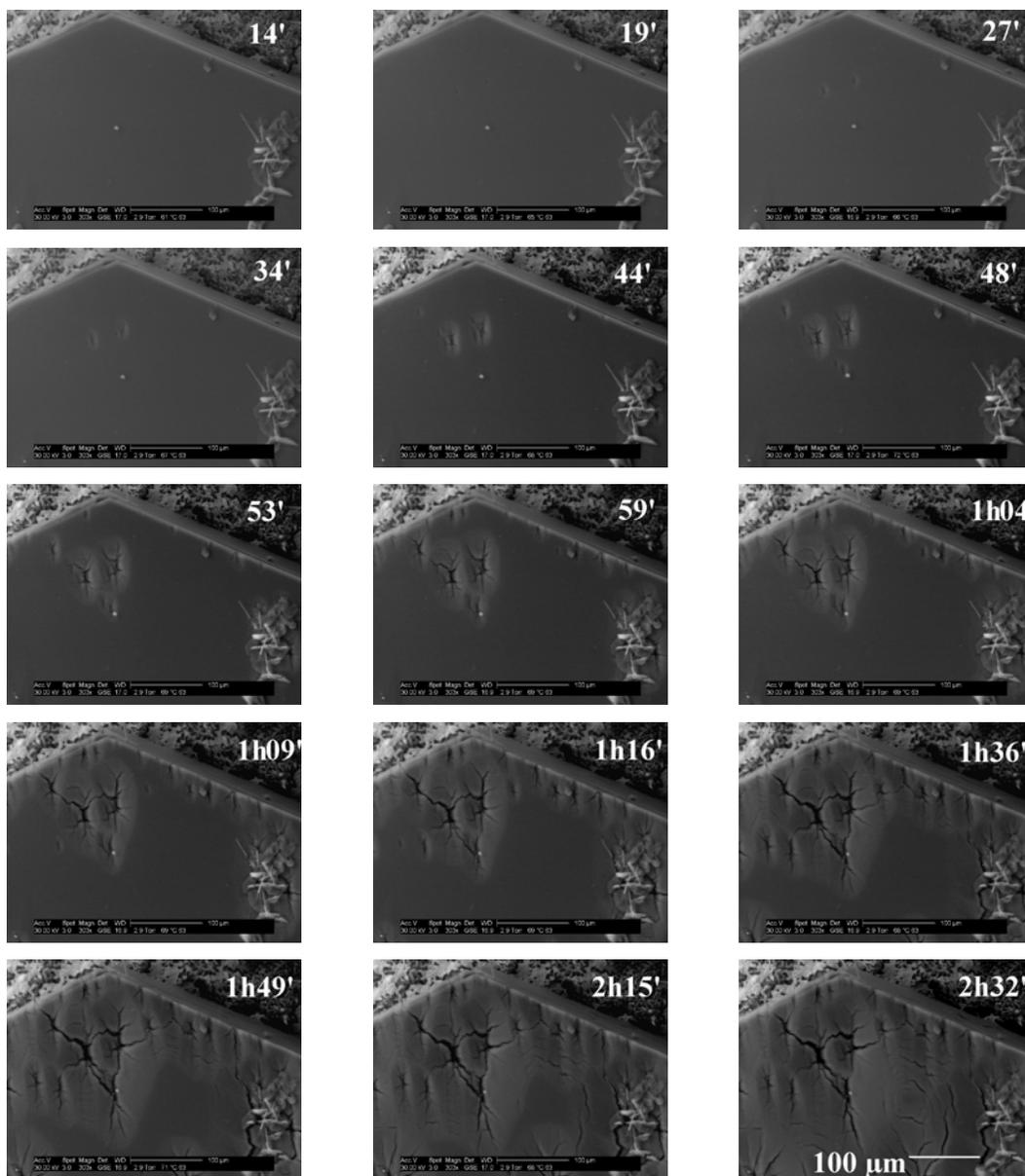
Fig. 5. Views of a  $\text{Li}_2\text{SO}_4 \cdot \text{H}_2\text{O}$  single crystal during dehydration with the environmental scanning electron microscope ( $T=70^\circ\text{C}$ ,  $P(\text{H}_2\text{O})=3.9$  hPa).
