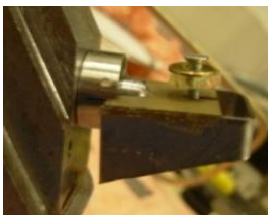
Fig. 2. Nozzle with deflector
