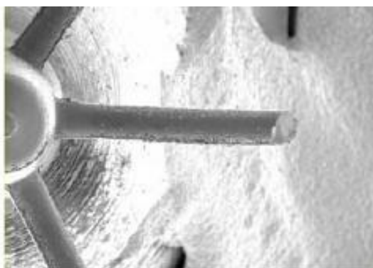
Fig. 1. Silicone mould of injector
