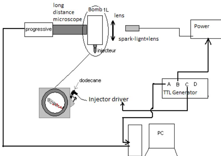
**Fig. 3** Experimental setup of the granulometry by imagery
