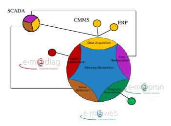
Figure 4. Blocks of ISO 13374-2 in the software suite of e-m@systec
