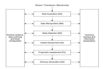
Figure 2. Data processing block diagram - ISO 13374-2 [10]
