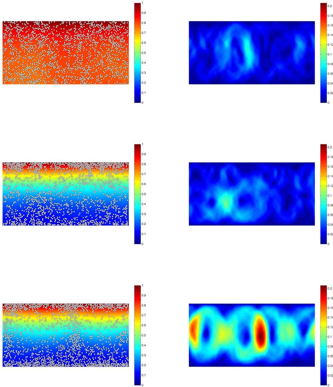
Figure 11: Dense suspension and oxygen distribution in a rectangular domain (l) and modulus of the velocity fluid (r) at different time steps  $t_n = n\Delta t$ . From top to bottom  $n = 3, 99, 1231$ .
