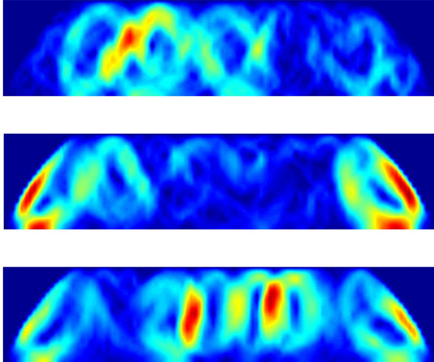
Figure 13: Modulus of the fluid velocity for a dense suspension in a drop domain at different time steps  $t_n = n \cdot \Delta t$ , for  $n = 3, 200, 350$
