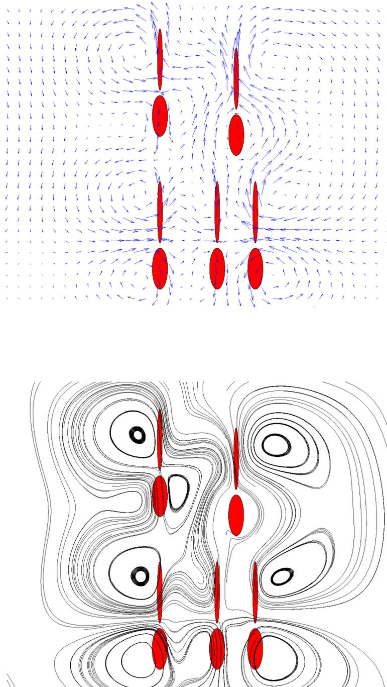
Figure 7: Velocity profiles ((a) velocity field (b) streamlines) in the fluid flow in the neighbourhood of five ellipsoidal bacteria interacting through the fluid flow
