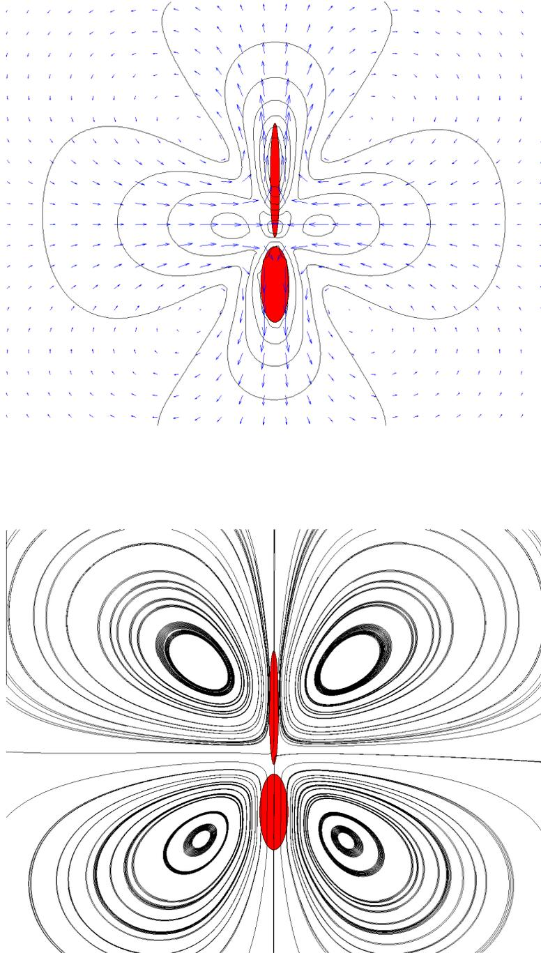
Figure 2: Velocity profiles ( (t) velocity field (b) streamlines ) in the fluid flow in the neighbourhood of an ellipsoidal bacterium
