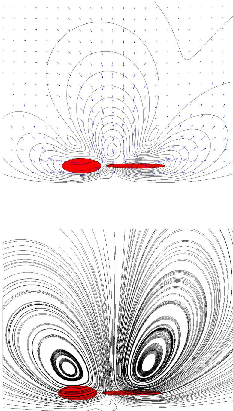
Figure 3: Velocity profiles ((t) velocity field (b) streamlines) in the fluid flow in the neighbourhood of an ellipsoidal bacterium located near a solid wall
