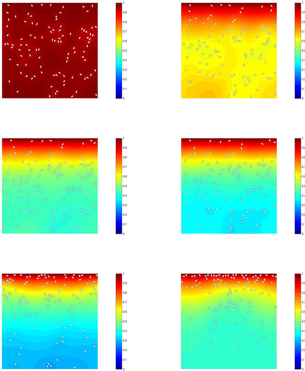
Figure 10: Position of 100 bacteria and oxygen distribution at different time steps  $t_n = n\Delta t$ . From left to right and from top to bottom :  $n = 1, 10, 20, 40, 50, 1000, 3400$ .
