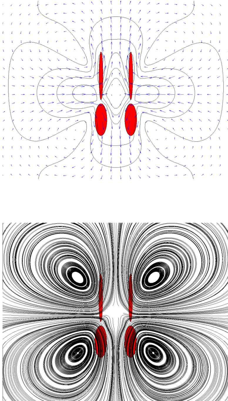
Figure 5: Velocity profiles ((t) velocity field (b) streamlines) in the fluid flow in the neighbourhood of two ellipsoidal bacteria interacting through the fluid flow
