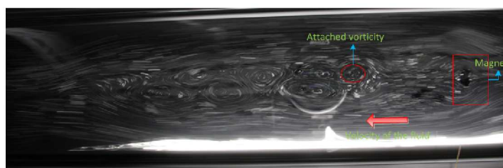
Figure 4: A street of vortices at Re = 1500
