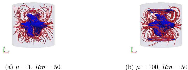
Figure 1: Magnetic lines and iso-value of the magnetic energy density corresponding to 25% of the maximum magnetic energy for two disks with different magnetic permeability \mu .
