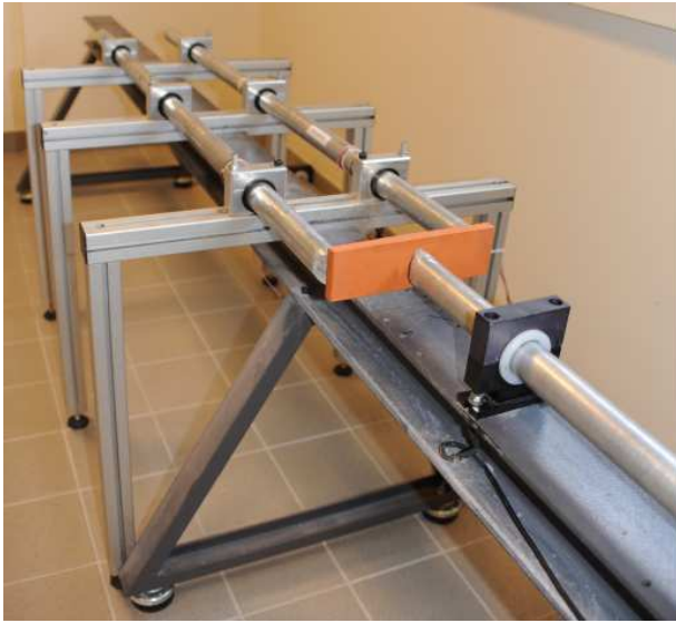
Figure 2: Photographs of the bending test set-up, brick specimen
