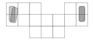
Fig. 7. HRP-2 experiment scenario. On the left, the vertical rectangle is the planned starting point and the rotated rectangle is the real starting point. On the right, the goal point which is reached independently of the initial error.
