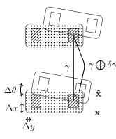
Fig. 3. Correction of the next step due to a position error of the robot waist. Dotted rectangles are the planned positions  $\mathbf{x}$  of the robot waist before and after the next step. Non-dotted rectangles corresponds to the robot real positions  $\hat{\mathbf{x}}$ . Error w.r.t to axis X, Y and yaw rotation is  $(\Delta x, \Delta y, \Delta \theta) = \delta \mathbf{x}, \gamma$  the reference trajectory and  $\delta \gamma$  the corrected trajectory reaching the planned step.
