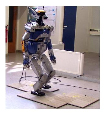
Fig. 1. HRP-2 robot following a trajectory in a constrained environment. In this experiment, the robot starting position is deliberately perturbed. During the execution, the correction algorithm automatically cancels the perturbation and the robot reaches the desired final position.
