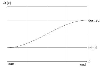
Fig. 4. Polynomial curve  $\Delta(t)$  providing a smooth transition between feet and center of mass trajectories.
