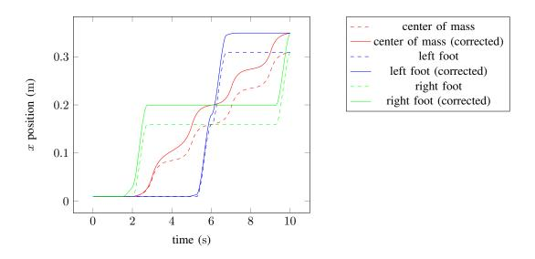
Fig. 5. Evolution, during two steps, of the x position of the center of mass and left foot. Solid curve depicts a step a 0.3m forward. Dashed curve depicts this step with a correction of 0.05m in the forward direction.
