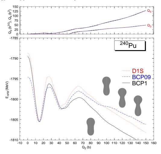
Figure 6. (Color online) In the lower panel the potential energy curve as a function of the quadrupole moment  $Q_2$  for the two BCP functionals and Gogny force used in the calculations is shown. In the upper panel, the octupole and hexadecapole moments are displayed again for the three interactions/force used. The lines lie on top of each other and are hardly distinguisable. See text for further details.
