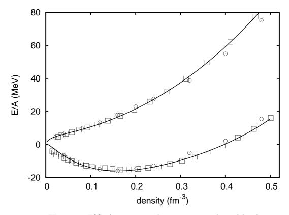
**Figure 1.** EOS of symmetric and neutron matter obtained by the microscopic calculation (squares) and the corresponding polynomial fits (solid lines). For comparison the microscopic EOS of Refs. [27] are also displayed by open circles
