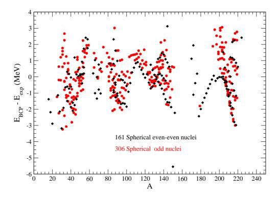
**Figure 4.** (Color online) Energy differences as a function of mass number for a set of 161 spherical nuclei (black points) and 306 spherical odd nuclei (red points).
