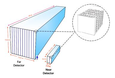
Figure 13. Sketch of the NO $\nu$ A detectors. The insert figure shows the plane arrangement of each detector. From [166].
