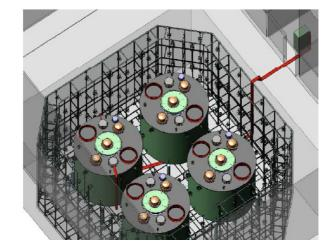
Figure 8. A drawing of the Daya Bay far detector hall showing the four detectors in a water pool instrumented with PMTs to detect cosmic muons. From [20].
