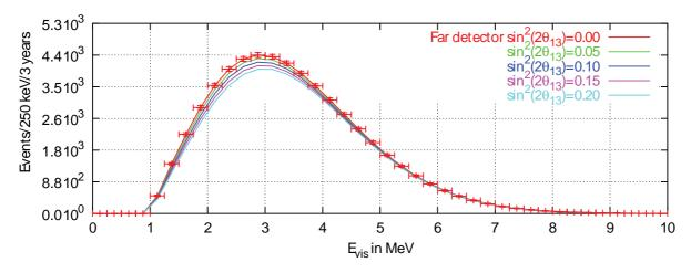
Figure 4. Neutrino induced positron spectrum for various values of  $\sin^2 2\theta_{13}$  simulated for the Double Chooz far detector [143].
