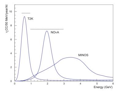
Figure 9. Muon neutrino interaction rates in MINOS, NO $\nu$ A, and T2K assuming no oscillations, normalised to one year of operation at the power of 410, 700, and 750 KW, respectively. The horizontal dotted lines represent the neutrino energy region where the  $\nu_{\mu} \rightarrow \nu_{e}$  oscillation probability is bigger than 50% of the maximum ( $\delta = 0$  and normal hierarchy). The MINOS probability is very similar to NO $\nu$ A.
