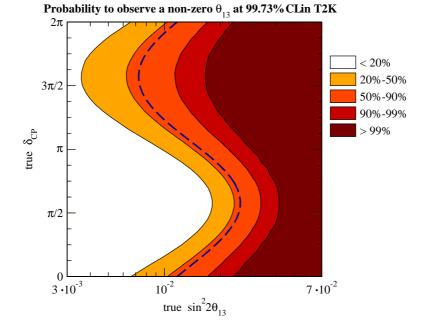
Figure 22. Contours of the probability  $P_{\text{disc}}$  to establish a non-zero value of  $\theta_{31}$  at the 99.73% CL for T2K in the  $\sin^2 2\theta_{13}^{\text{true}} - \delta^{\text{true}}$  plane. The dashed curve corresponds to the "standard sensitivity limit". Reprinted from Ref. [181], Copyright (2007), with permission from Elsevier.
