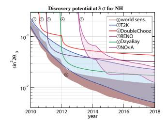
Figure 20. Evolution of the  $\theta_{13}$  discovery potential as a function of time (3 $\sigma$  CL) for NH, showing the global sensitivity reach. The bands for the beams and the global reach reflect the (unknown) true value of  $\delta$ . For Daya Bay we have assumed a systematical uncertainty of 0.38% correlated among detector modules at one site.
