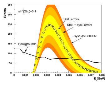
Figure 5. Number of disappeared events in Double Chooz for  $\sin^2 2\theta_{13} = 0.1$ , i.e., the difference between no-oscillation and oscillation spectra in the far detector, compare fig. 4. Also shown are statistic and expected systematic errors, together with systematic errors as big as the former Chooz experiment. The signal is compared to the expected background rate. Based on data from [21].
