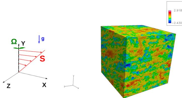
Figure 1: Sketch of the mean flow (left). Buoyancy distribution (right). DNS with  $512 \times 768 \times 512$  degrees of freedom with Richardson number  $Ri = 0.5$  and baroclinicity parameter  $\varepsilon = 0.2$ .  $Re_\lambda(0) = 44.1$  and  $\frac{Sk}{\varepsilon_\nu} = 2.55$ . With  $\varepsilon_\nu$  the kinetic energy dissipation.  $\tau = tS = 7$ .
