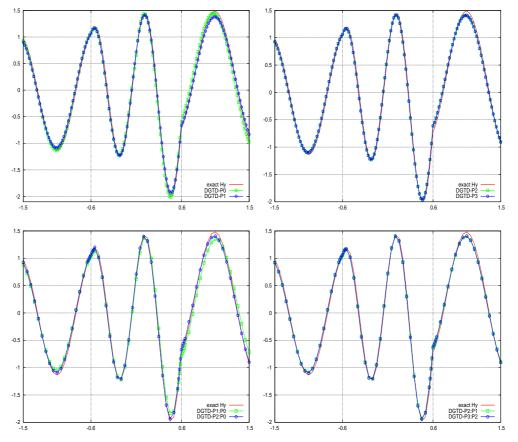
FIGURE 4.12. Scattering of a plane wave by a dielectric cylinder. 1D distribution of  $H_y$  along y = 0.0 at time t = 5. DGTD- $\mathbb{P}_p$  method (top) and DGTD- $\mathbb{P}_{p_c}$ : $\mathbb{P}_{p_f}$  (bottom).
