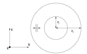
FIGURE 4.1. Concentric PEC cylinders resonator setting.
