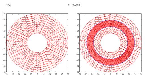
FIGURE 4.2. Concentric PEC cylinders resonator. Example of conforming (left) and non-conforming (right) triangular meshes.
