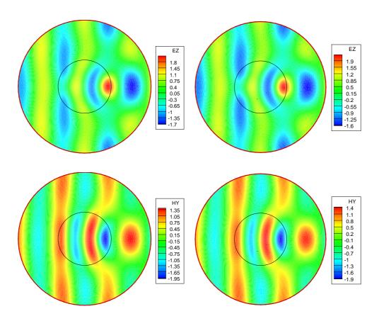
FIGURE 4.10. Scattering of a plane wave by a dielectric cylinder. Contour lines of  $E_z$  (top) and  $H_y$  (bottom) at times t = 1 (left) and t = 10 (right). DGTD- $\mathbb{P}_1$  method using a conforming mesh with 6001 nodes and 11920 triangles.
