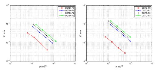
FIGURE 4.7. Rectangular PEC resonator with material interface. Numerical convergence of the *h*-refinement DGTD- $\mathbb{P}_p$  method. Conforming (left) and non-conforming (right) triangular meshes.
