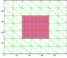
FIGURE 3.2. Non-conforming locally refined triangular mesh.
