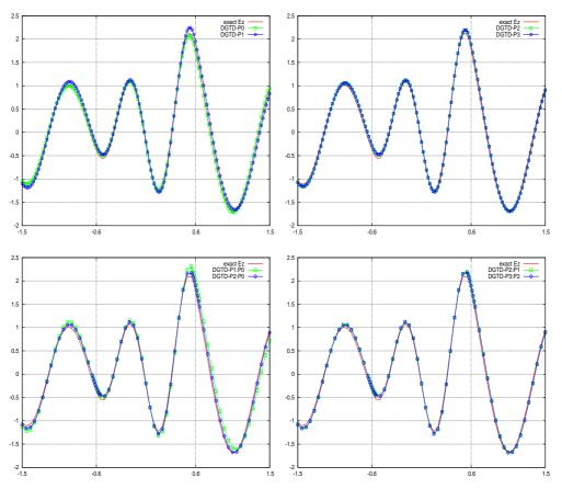
FIGURE 4.11. Scattering of a plane wave by a dielectric cylinder. 1D distribution of  $E_z$  along y = 0.0 at time t = 5. DGTD- $\mathbb{P}_p$  method (top) and DGTD- $\mathbb{P}_{p_c}$ : $\mathbb{P}_{p_f}$  (bottom).
