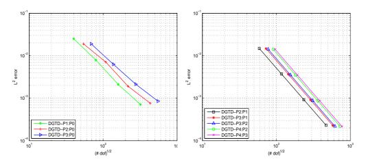
FIGURE 4.5. Concentric PEC cylinders resonator. Numerical convergence of the  $hp\text{-refinement DGTD-}\mathbb{P}_{p_c}{:}\mathbb{P}_{p_f}$  method. Non-conforming triangular meshes.
