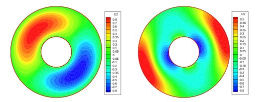
FIGURE 4.3. Concentric PEC cylinders resonator. Contour lines of  $E_z$  (left) and  $H_y$  (right) at time t = 10. DGTD- $\mathbb{P}_1$  method using a conforming mesh with 1088 nodes and 2048 triangles.
