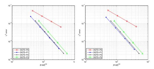
FIGURE 4.4. Concentric PEC cylinders resonator. Numerical convergence of the *h*-refinement DGTD- $\mathbb{P}_p$  method. Conforming (left) and non-conforming (right) triangular meshes.
