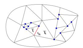
FIGURE 2.1. Irregular mesh with hanging nodes.
