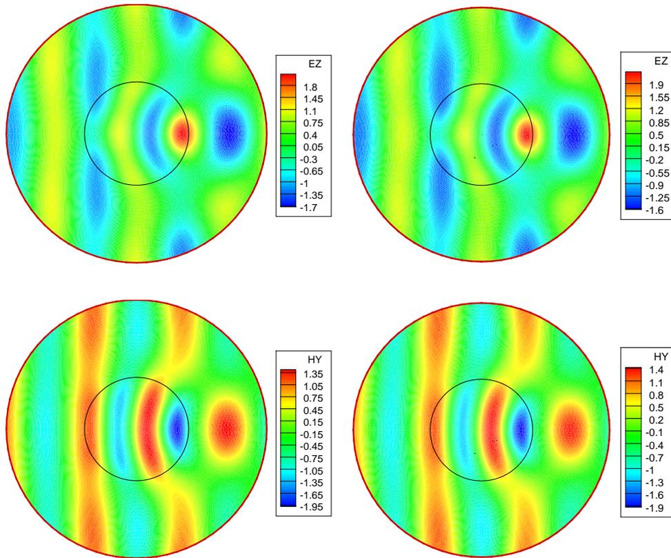
FIGURE 4.10. Scattering of a plane wave by a dielectric cylinder. Contour lines of  $E_z$  (top) and  $H_y$  (bottom) at times  $t = 1$  (left) and  $t = 10$  (right). DGTD- $\mathbb{P}_1$  method using a conforming mesh with 6001 nodes and 11920 triangles.
