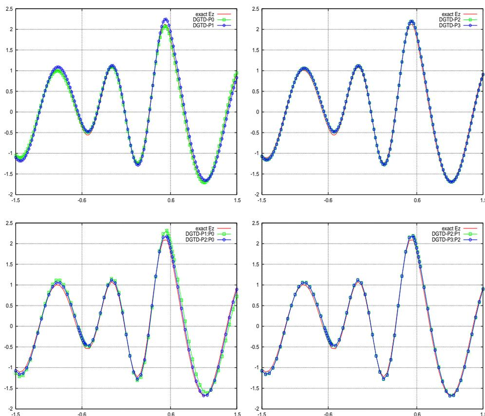
FIGURE 4.11. Scattering of a plane wave by a dielectric cylinder.
