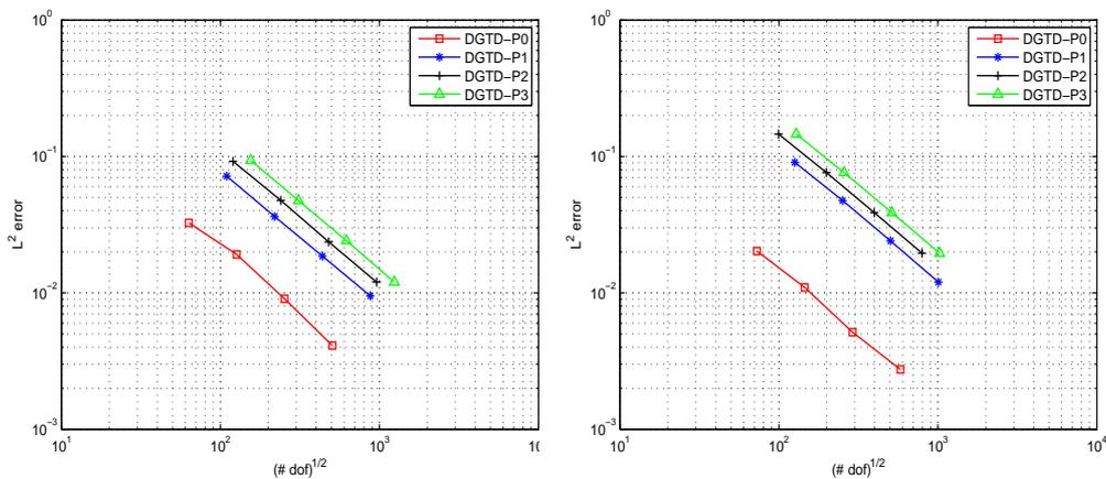
FIGURE 4.7. Rectangular PEC resonator with material interface. Numerical convergence of the  $h$ -refinement DGTD- $\mathbb{P}_p$  method. Conforming (left) and non-conforming (right) triangular meshes.
