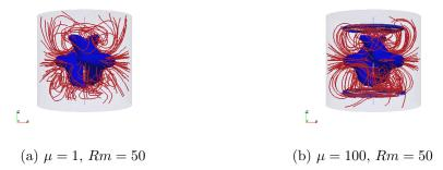
Figure 1: Magnetic lines and iso-value of the magnetic energy density corresponding to 25% of the maximum magnetic energy for two disks with different magnetic permeability  $\mu$ .
