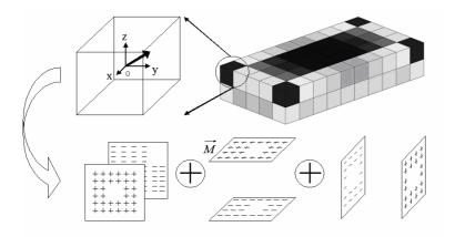
Fig. 4. Surface charge method to compute torque when magnetization of each bloc is known.
