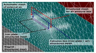
Fig. 6. Difficult mesh in 3D FEM software Flux3D<sup>TM</sup>
