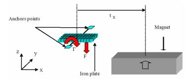
Fig. 2. Magnetic MEMS topology
