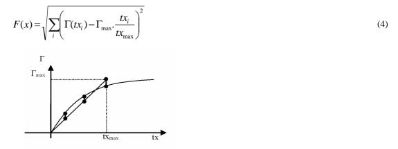
Fig. 3. Design specification: torque has to be linear
