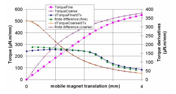
Fig. 9. Fine and coarse torques and their formal derivatives, versus the magnet translation.
