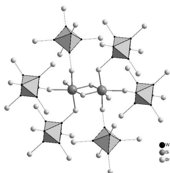
Figure 2. Connectivity of (\text{BiBr}_2)_2 units with outer bromide cluster ligands. (\text{W}_6\text{Br}_8^i) clusters are shown as octahedra.
