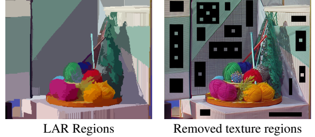
Figure 2: Adapted regions, black regions are removed to be synthesized at decoder side.
