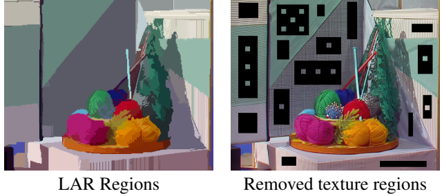
Figure 2: Adapted regions, black regions are removed to be synthesized at decoder side.
